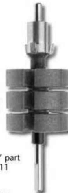
The XXX Slotted armature was designed to exploit the increased magnetic field of the D3's new 6.0v wet magnets and innovative can design. This combination of XXX armature and D3 setup makes for a more efficient motor without sacrificing top end. The D3 produces the same torque as the older D2 motors but with an increase of usable rpm. The power band has also been widened to make the D3 more drivable over a wide variety of track and car conditions.
