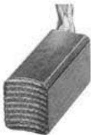
"L" Slot brushes have a slot running from top to bottom. This slot helps the brush center itself on the commutator, and cleans the commutator while running.
