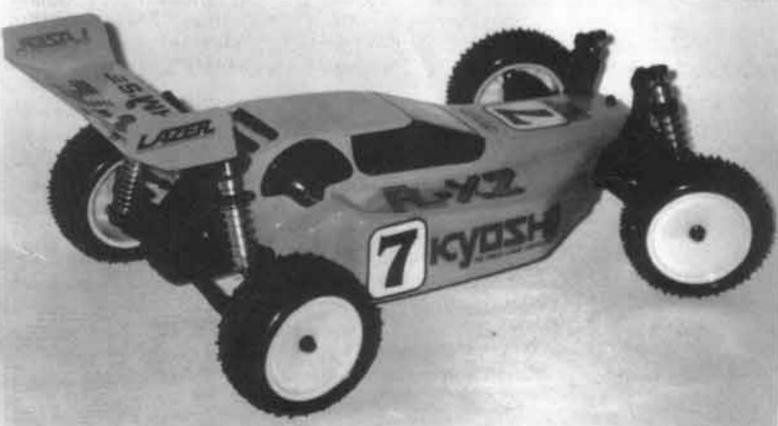
**D150 RAZER™** DAHM'S RAZER Body fits the Kyosho Lazer, Raider Pro, and Yokomo YZ10. RAZER features narrow aerodynamic styling, trim lines, rear vents, motor cooling vents that can be cut open, and a Super Fin Wing™. Use Power Pan Underbody No. D155 with the RAZER.
