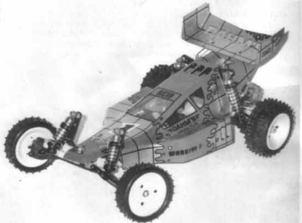
**D170 WARRIOR II™** The WARRIOR II Body fits the RC10 and RC10 Graphite. WARRIOR II features include low, aerodynamic styling, shock tower bracing, wide side pods, cooling vents, and a Super Fin Wing™. Use Power Pan Underbody No. 175 with this body.
